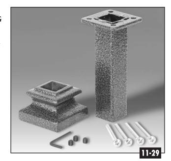
Begin installation by drilling or cutting a hole in the proper location. With the base collar placed on the newel, attach the shaft to the precut newel with the provided allen wrench and screws. **PHOTO 11-30.**
